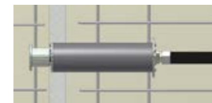
Embedment jointmeter installation scheme
