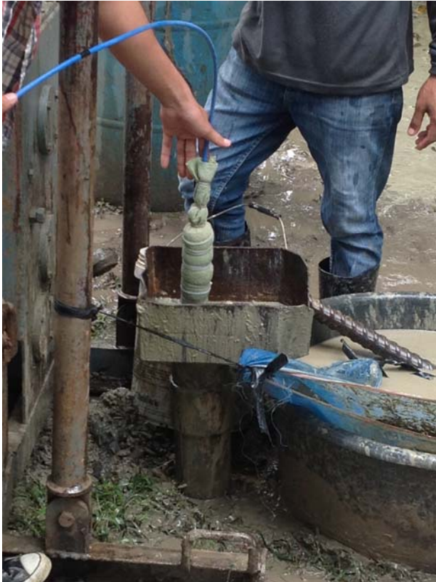
Insert the transducer in the borehole
