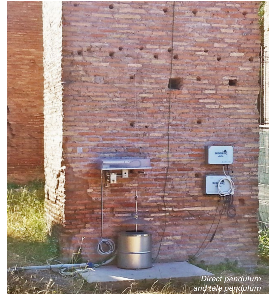
Digital tilt meter installed on Maxentius Basilica
