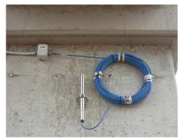
They provide a direct measure of the effect on the structure of complex process as for example the soil consolidation with related differential settlement, sand liquefaction, water table variation, etc.
