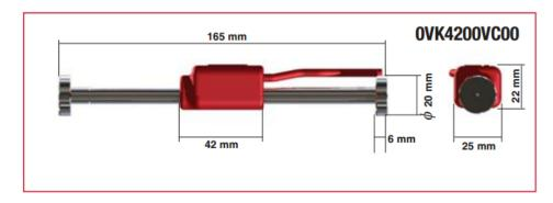
Deformation of the structure will cause the two end blocks to move relative to each other, thus altering the tension of the steel wire.
